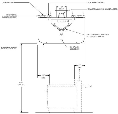
The amount of exhaust volume required is dependent upon the type of cooking equipment and the type and volume of cooking. Contact factory for exhaust volumes, duct sizes, and static pressures.
